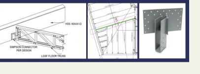
The HHSUQ is a high-load, face-mount, truss-to-truss hanger designed to accommodate severe skews (45°-84°) for hip trusses, enabling a greater range of installation applications. Fastening the HHSUQ with Strong-Drive® SDS Heavy-Duty Connector screws makes installation fast and easy, while eliminating the inconvenience of bolted applications. As per the plan geometry the building is not perfectly 90° so as the trusses.
